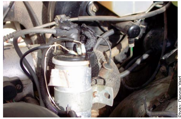
Photo: Lucas coil leaking black tar
