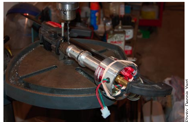
Photo: Step 10 - Drilling the shaft for the gear pin
